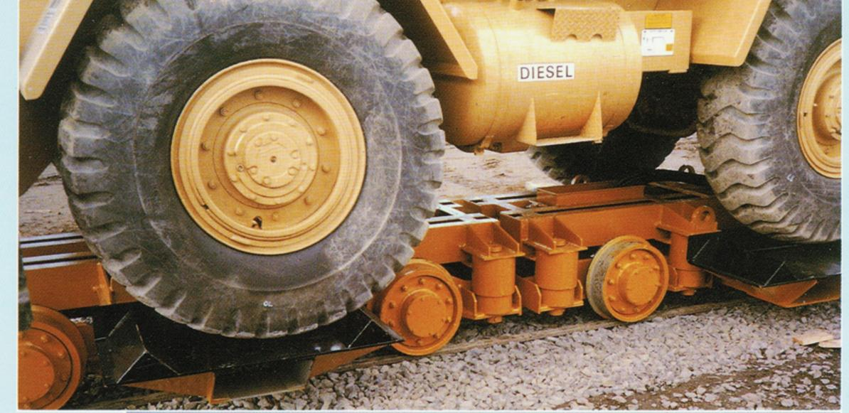
Custom built bogies, along with insulated wheel options are offered in a range of sizes, depending on tare weights, track gauges and insulation requirements.
